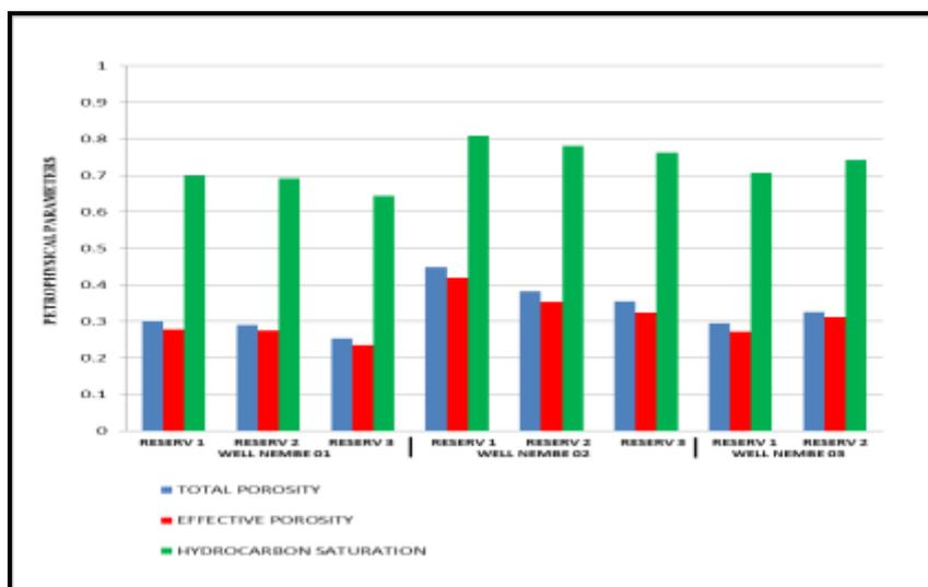
**Figure 10:** Combined Bar chart showing Variations of Reservoir Properties in Well NEMBE 01, 02 & 03
