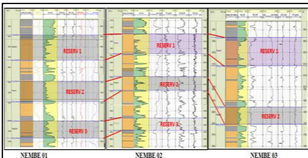
**Figure 2:** Wells NEMBE 01, 02 and 03 showing Suite of Logs, Delineated Lithology and Reservoirs 1, 2 and 3
